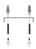
2. Apply screws into plastic anchors
