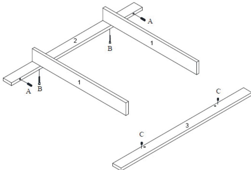
**Step 4.1 :** Use both barriers **1**, the cross-bars **2** and **3**, two wooden dowels **A**, two wood screws **B** and two pvc nuts **C**
