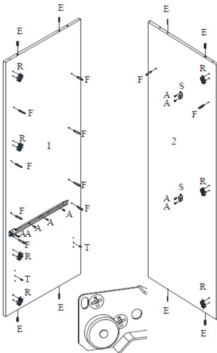
**Step 4.1 :** Use the left side **1**, the right side **2**, eight wooden dowels **E**, ten connectors **F**, one slider **L**, seven hinge mounting plates **R**, two rod holders **S**, nine wood screws **A** and two shelf supports **T**
