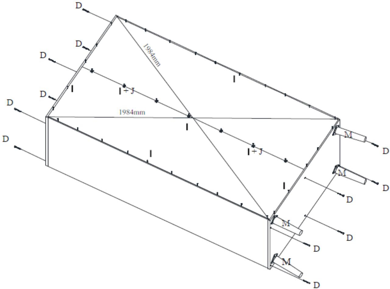
**Step 4.8 :** Use the parts from step 4.3 and step 4.4, the construction from step 4.7, twelve wood screws **D**, both backs **18**, seven panel clamps **J** and thirty-seven wood screws **I**.
