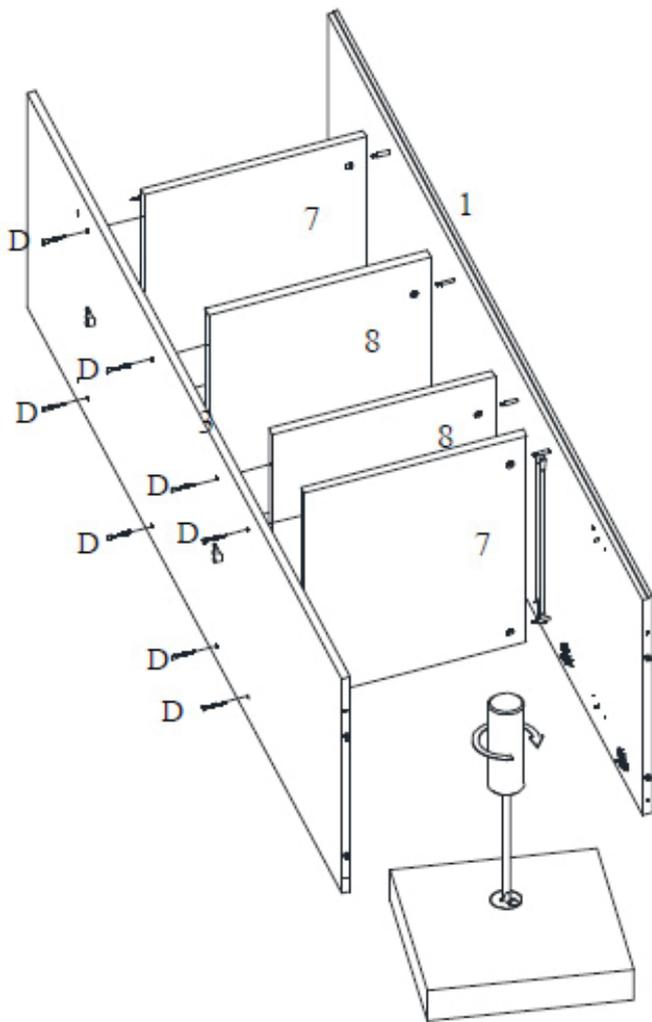
**Step 4.6 :** Use the shelves **7** and **8** of step **4.5**, the left side of step **4.1**, the intermediate side of step **4.2** and eight wood screws **D**
