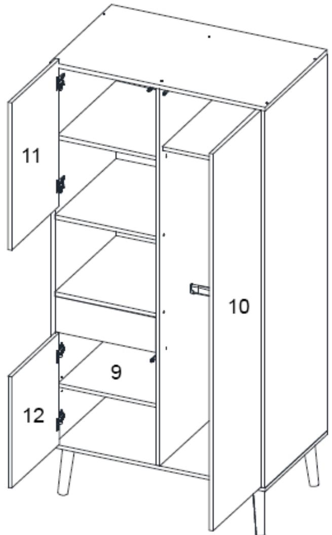
**Step 4.12** : Use the cupboard structure from step 4.8, the doors from step 4.11, the drawer from step 4.10, both **clothes bars** and the mobile shelf 9.
