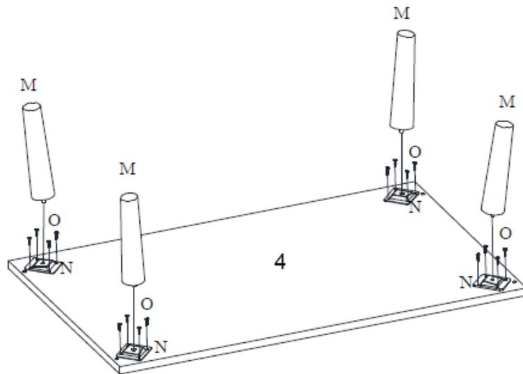
**Step 4.4 :** Use the bottom **4**, the four legs **M**, four mounting plates **N** and sixteen wood screws **O**.
