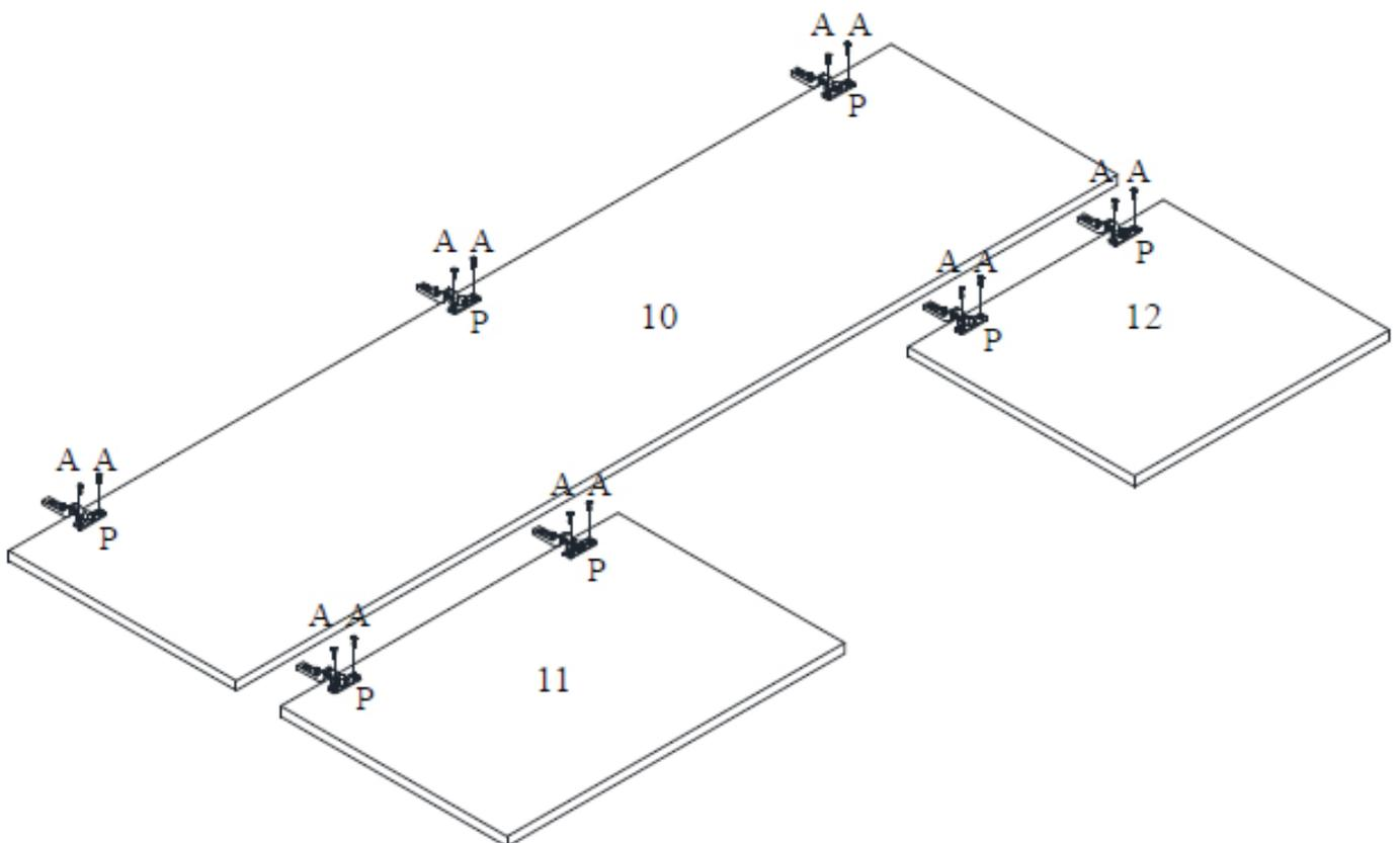
**Step 4.11 :** Use the doors **10**, **11** and **12**, seven hinges **P** and fourteen wood screws **A**
