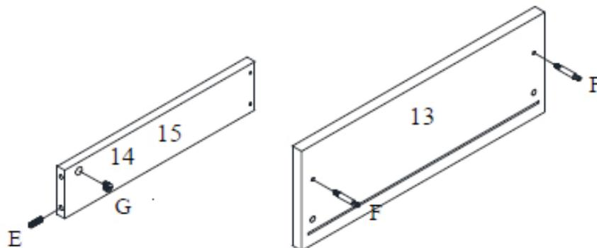
**Step 4.9 :** Use the drawer front **13**, the drawer sides **14** and **15**, two connectors **F**, two wooden dowels **E** and two minifix **G**
