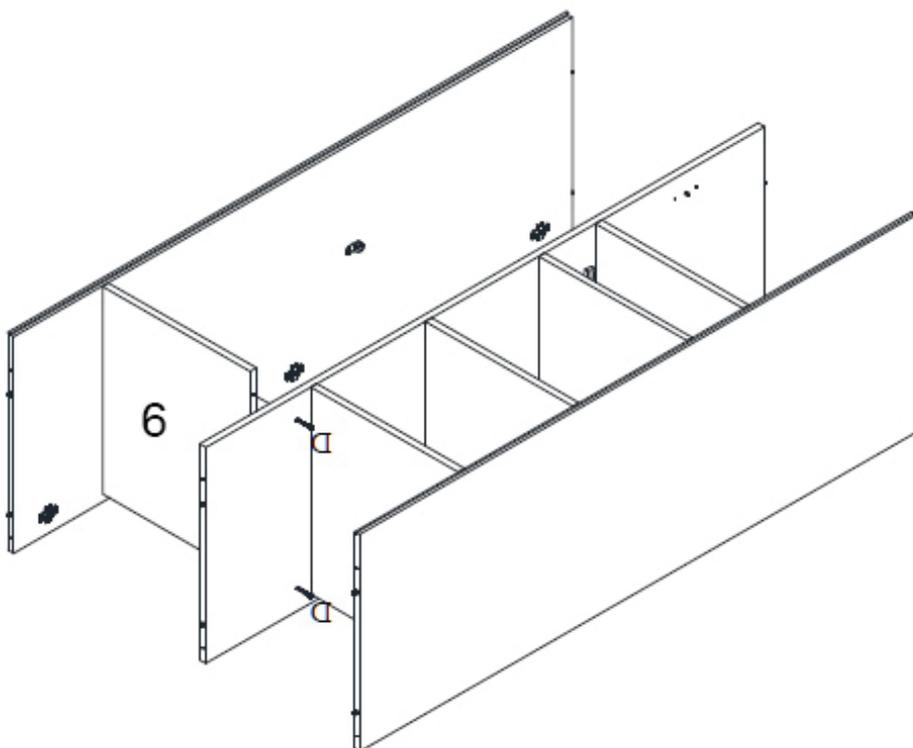
**Step 4.7 :** Use the parts from step **4.6**, the shelf **6** from step **4.5**, the right side of step **4.1** and two wood screws **D**
